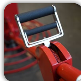
Quick pull wing adjustment
