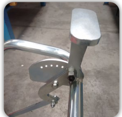
Dosage setting from 1 to 6 \text{ kg/m}^2
