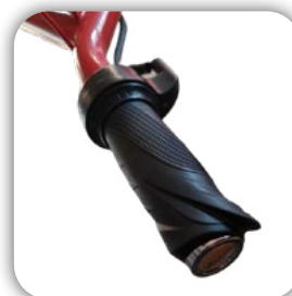
Hand throttle for stepless speed control
