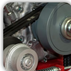
Automatic V-belt tensioner for permanent tensioned V-belts
