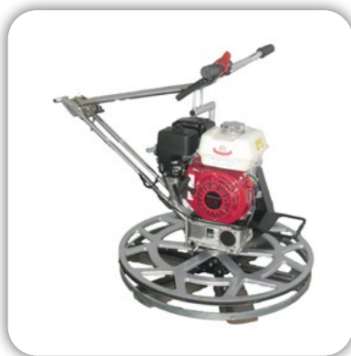
Folding drawbar for compact and easy transport
