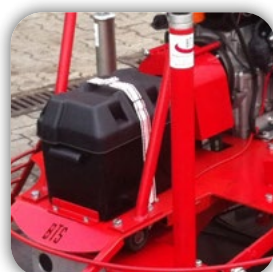
Battery box for permanent protection of the battery
