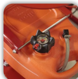
Plastic fuel tank with fuel gauge
