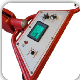
11 inch display with battery indicator and remaining driving time
