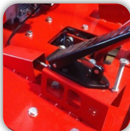
Gas pedal stepless adjustment 40-180 rpm
