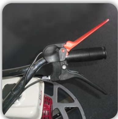
2 in 1 dead man's switch with gas handle for easy handling
