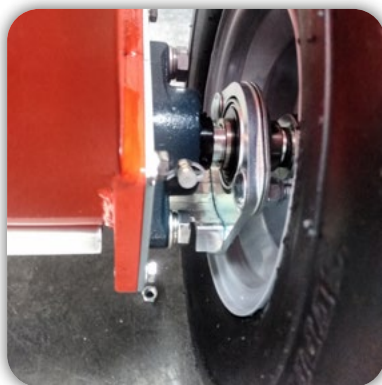
Cast iron bearings for high sliding stability
